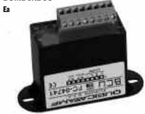
This box enables Qubica scoring systems to raise and lower automatic bumper systems automatically.
