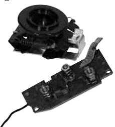
The "small disk" mechanism and switch for starting early model Westinghouse BE motors.
