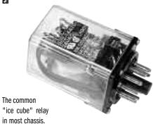
In the SS chassis, SP relay 070 005 883 looks very similar, but it has a 10 VCC coil and is not interchangeable.
