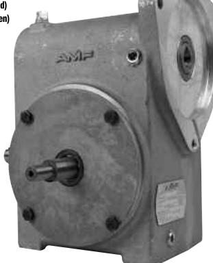
This gearbox design, used on 82/90 and later pinspotters, points the motor forward underneath the wireway.
