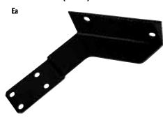
These brackets connect the sweep bar to the sweep shock mounts and don't use sliders like older versions
