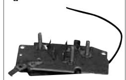
These two switches inside the top of Westinghouse Sweep & Table motors work together to engage the start windings of the motor.
