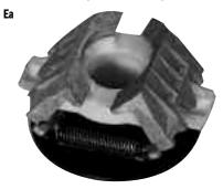
The "wide disk" mechanism and switch for starting late model Westinghouse and A.O. Smith BE motors.
