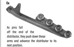
Bearings that are missing or that don't spin freely should be replaced with Bearing 000 026 251BG, Screw 813 540 082BG, and Lockwasher 957 100 002BG.
